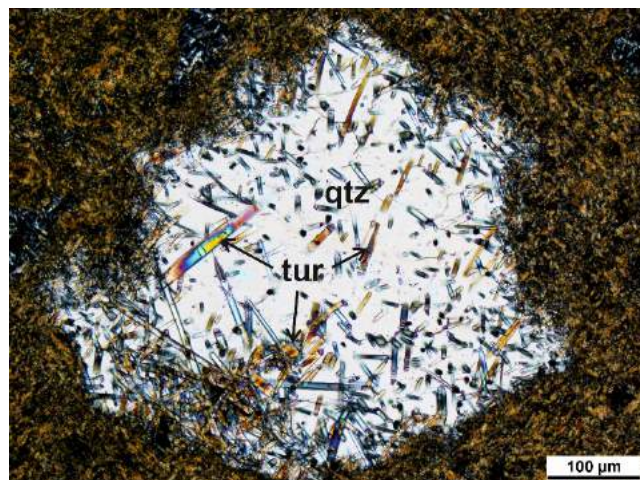
Figure 2. Idiomorphic tourmaline (colourful prism) growing into quartz (white) within subhedral masses of tourmaline, finely intergrown with chlorite. These minerals occur associated with several of the mineralisation stages.
