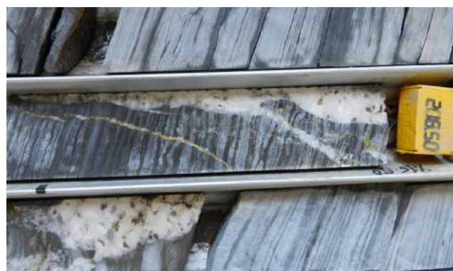
Figure 2. Late orogenic Lufilian veins bearing Cu-Co sulfides (chalcocite, chalcopyrite and carrollite \pm bornite) in the lower ore body (drill hole KAMA0052, HQ core samples 64 mm wide).
