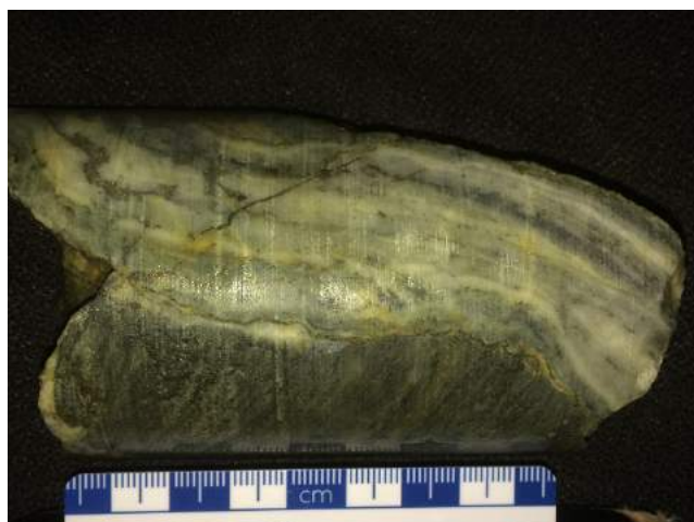
Figure 5. Photo of core from drill hole KG-10 intersecting auriferous banded quartz vein at the Kilmacoo deposit. The specimen shows a distinct cross-cutting relationship between the banded silica and an early Caledonian penetrative cleavage ( S_1/S_2 ), confirming a late paragenesis for gold at Kilmacoo.
